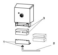
Insert smaller foam gasket (3) into the strain relief. Install solenoid cable plug (1) into the smaller, telephone-style jack in the transformer. Install faucet sensor cable plug (2) into the larger RJ-45 jack.
